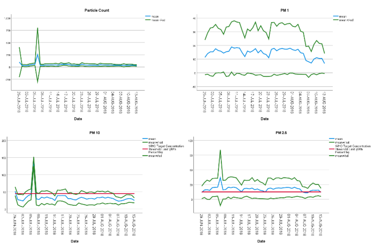
Figure 1: Daily averages, Upper bounds, Lower bounds and WHO target concentration for Particle count, PM1, PM2.5, and PM10.
