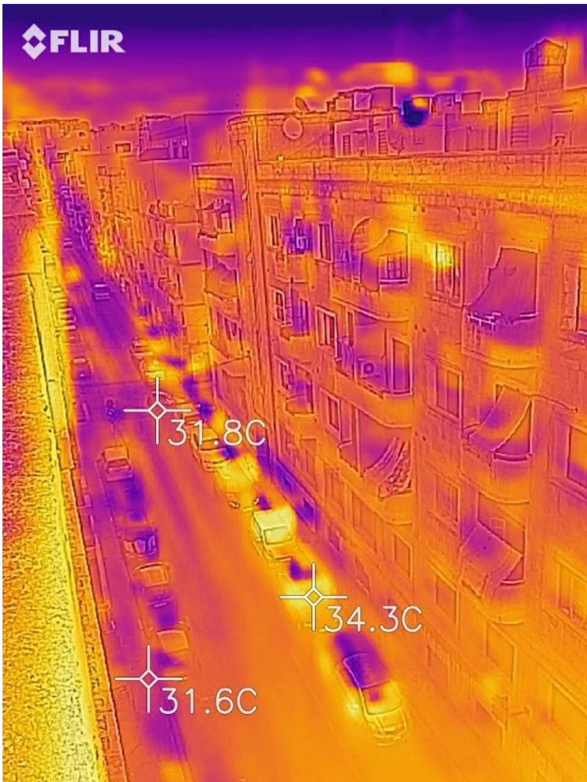
Figure 5: Triq D'Argens, Gzira (shaded from the sun) remaining warmer than the nighttime ambient temperatures despite passing vehicles air drag that is presumed to cool the surfaces to ambient temperature. Taken in Triq D'Argens, Gzira on the 9th July 2019 07:00 hours.
