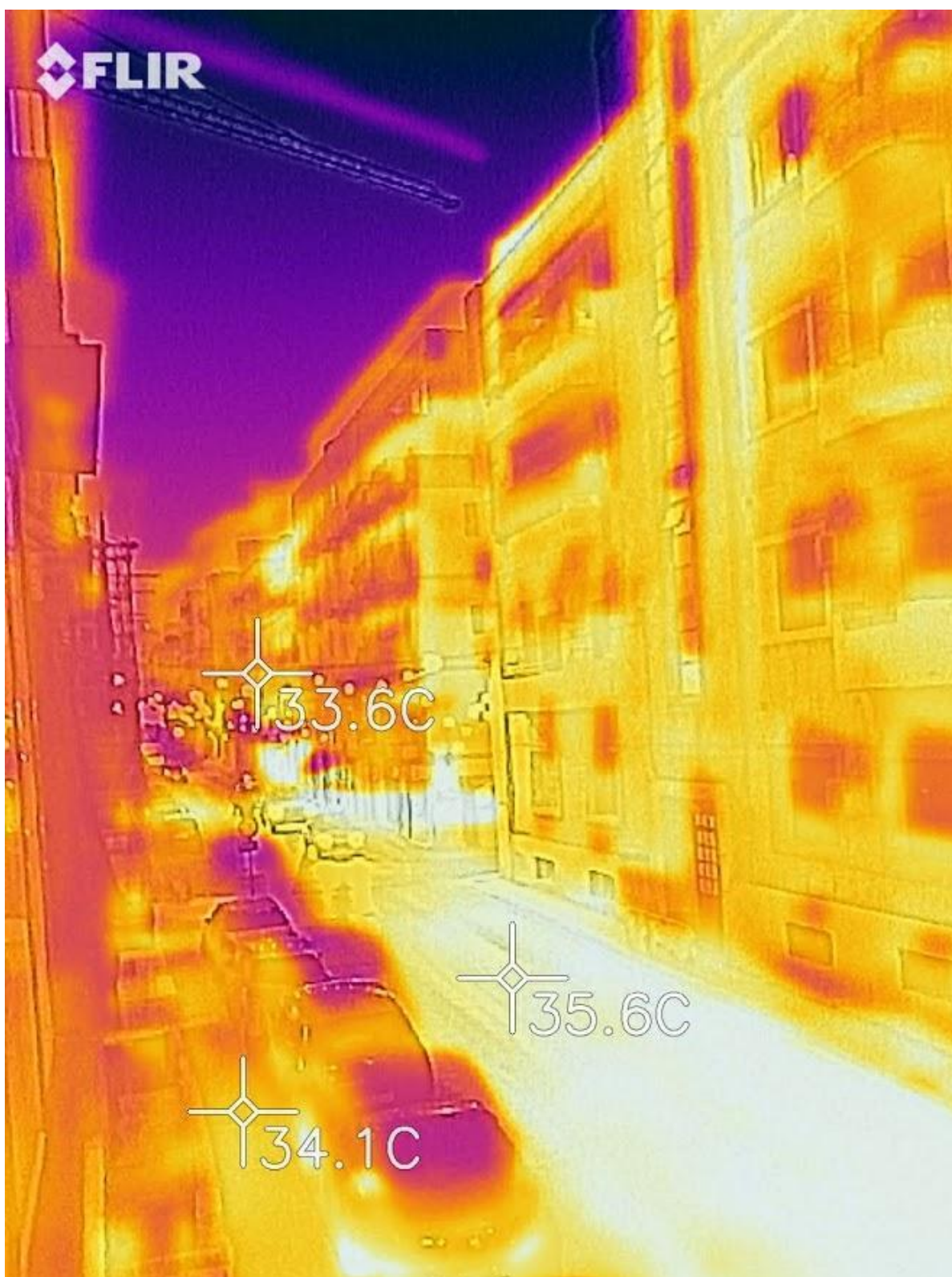
Figure 4: UHI heat entrapment throughout night, despite passing vehicles air drag that is presumed to cool the surfaces to ambient temperature. Taken in Triq D'Argens, Gżira on the 8th July 2019 21:00 hours.
